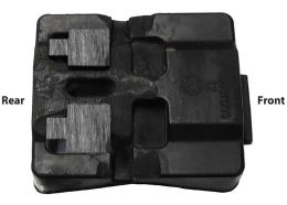
On used stops you may need to remove 1/16" or so from here until it sits flush with the rubber stop.
