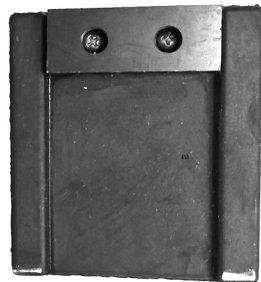
Top of right stop with shim installed
